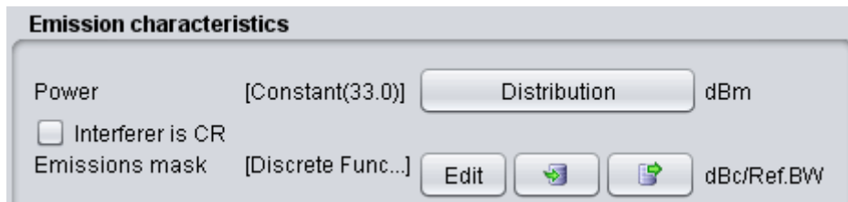
Figure 285: Example on how to import/export to/from the workspace/library for the spectrum emission mask
