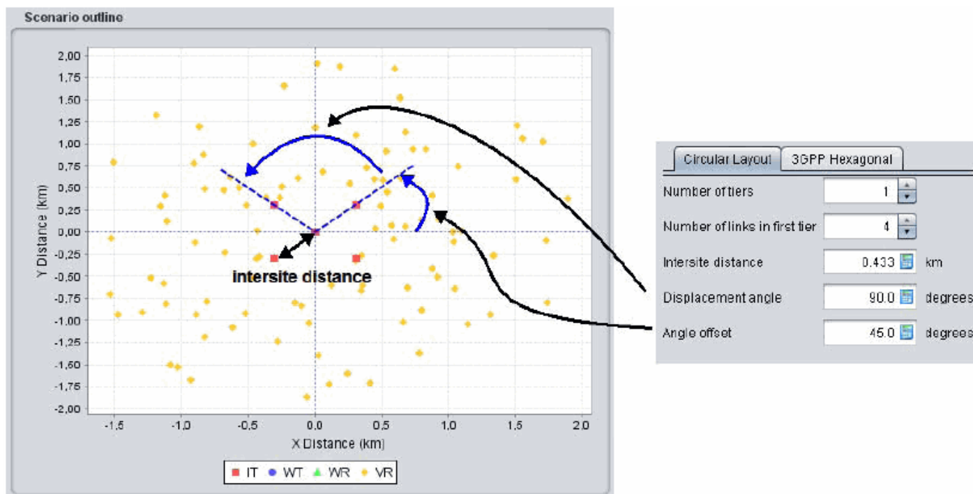
Figure 219: Example where 1 tier is used to position 4 interferers in a square shape (i.e. corners of a building) with the Vr positioned outside the square
